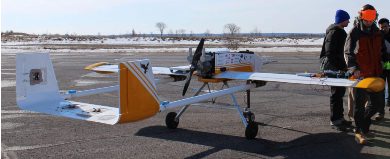
Figure 1 Photograph of the GeoSurv II. It is powered by a 2-stroke 22 kW engine.
